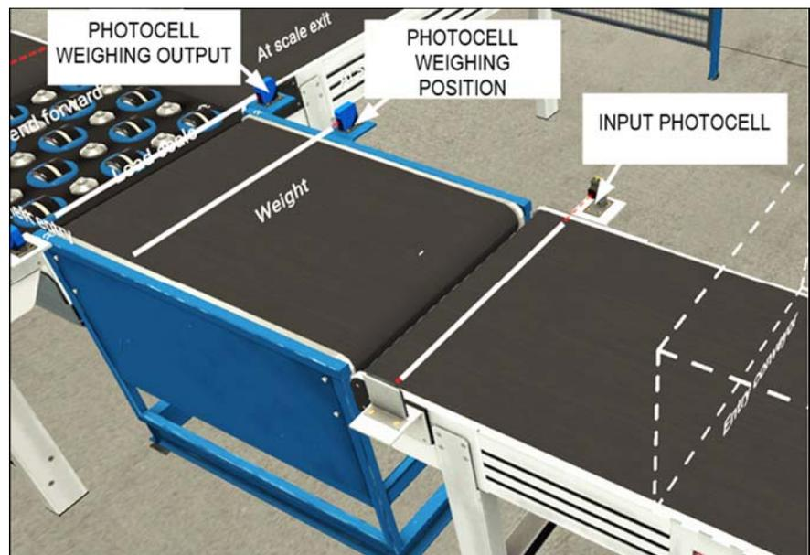
**Figure 4.** Detail of the conveyor belts and sensors in the layout
