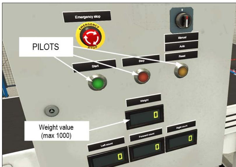
**Figure 5.** Detail of the layout's control panel
